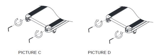
• Test for at least 15 seconds at 4km/h (check and adjust a further quarter or half turn until the belt is centred).
