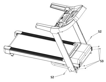
Step 1 Installing the upright frame
