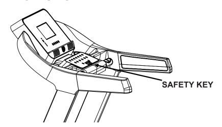
Before beginning a workout session ensure that the Safety Tether Key is properly placed onto the Computer Console and the Safety Clip is securely attached to an article of your clothing. If you fall the clip will pull out the SAFETY KEY from the Computer Console and the running belt will stop immediately for emergency stop, helping to prevent injury.
